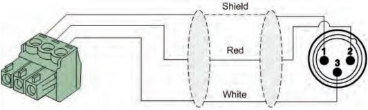
For unbalanced line input connections:
