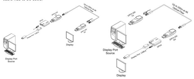
DPAX can improve transmission length of DPFX-250 via optical fiber. It has been confirmed that DisplayPort signal transmission length has improved up to 300m when using DPFX-250 with DPAX under certain environment such as below configuration. Each 200m and 300m of DisplayPort signal transmission has successfully tested when using GTX960 as a display source and ASUS PA328Q as a display.
