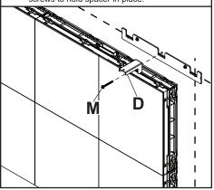
ENG For 5 ft. covers, install first bracket in the middle space, then every 12". Optional: Use wood screws to hold spacer in place.
