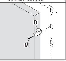
ENG For 6 - 8 ft. covers, install first bracket at the end space, then every 12". Optional: Use wood screws to hold spacer in place.
