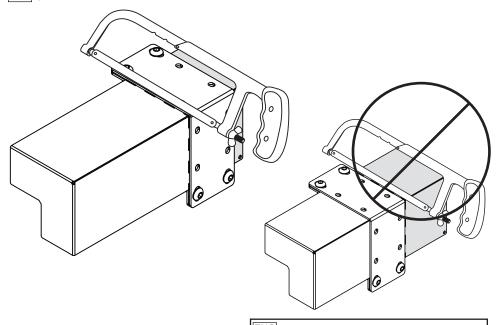
ENG Do not clamp fixture on wrong side of cutting line.
