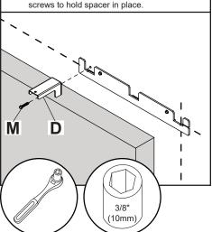
ENG For 6 - 8 ft. covers, install first bracket at the end space, then every 12". Optional: Use wood screws to hold spacer in place.
