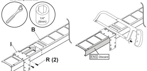
ENG Align bottom of spacer cutout and vertical notch with guiding lines.
