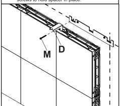
ENG For 6 - 8 ft. covers, install first bracket at the end space, then every 12". Optional: Use wood screws to hold spacer in place.
