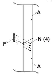
ENG Attach tooglers loosely, one at a time. Then, tighten all. Displays not shown for clarity.
