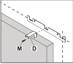
ENG For 5 ft. covers, install first bracket in the middle space, then every 12". Optional: Use wood screws to hold spacer in place.
