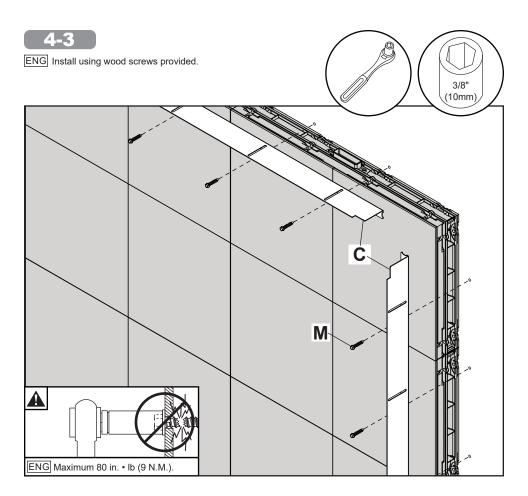
$\overline{\text{ENG}} \ \ \text{Slide wall brackets in slot until they sit 1.25" from display guiding lines. Level and tighten wood screws.}$
