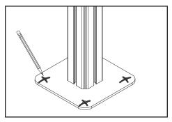
ENG Drill mounting holes into supporting surface (3" (76 mm) minimum depth required).
