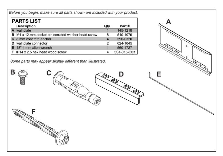
When installing additional wall plates (sold separately), attach two wall plate connectors (D) on either end of wall
