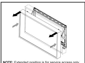
**NOTE:** Extended position is for service access only. The mount must be closed during normal use and operation.
