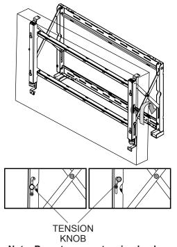
Note: Do not remove tension knobs.
