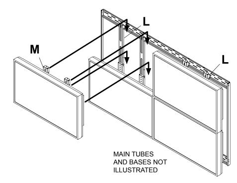
Secure top adapter brackets (M) to hook on **11)** brackets (L) using four M5 x 10 mm socket pin type-F screws (R) as shown below.
