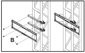
Use the outermost compatible hole positions to mount the plate supplied with separate mount and secure using taptite screws provided.
