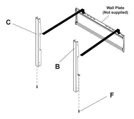
Secure adjustment brackets (**D**) to right and left vertical supports (**B** and **C**) using eight M5 x 16 mm phillips screws (**E**). Position right and left vertical supports (**B** and **C**) in desired location then tighten M5 x 25 mm phillips screws (**F**).
