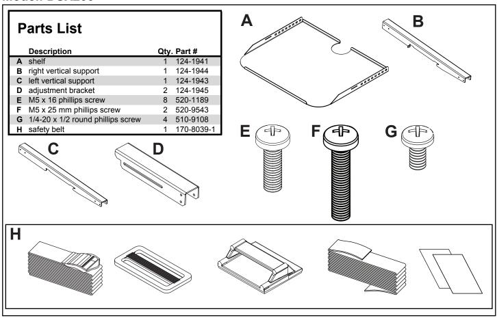
Secure two adjustment brackets (**D**) to shelf (**A**) using four 1/4-20 x 1/2 round phillips screws (**G**).
