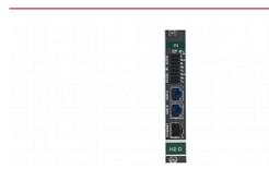
DTAxrD2-IN2-F34 is a 2-channel, 4K@60Hz (4:4:4), DSC, HDMI, analog audio, bidirectional RS-232, Ethernet, & IR over HDBaseT twisted pair receiver card for compatible Kramer Modular Multi-Format Digital Matrix Switchers. DTAxrD2-IN2-F34 inputs two extended-reach HDBaseT signals with selectable embedded/de-embedded analog audio, bidirectional RS-232, Ethernet, and IR from the line to the chassis
