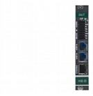
DTAxrD2-OUT2-F34 is a two-channel, 4K@60Hz (4:4:4), DSC, HDMI, analog audio, bidirectional RS-232, Ethernet, & IR over HDBaseT twisted pair transmitter card for compatible Kramer Modular Multi-Format Digital Matrix Switchers. DTAxrD2-OUT2-F34 outputs two extended-reach HDBaseT signals with selectable embedded/de-embedded analog audio, bidirectional RS-232, IR, and Ethernet from the chassis to the line
