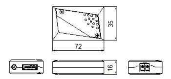
Note: The transmitter, HDFX-200-T and the receiver, HDFX-200-R have the same mechanical dimensions
