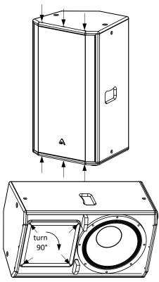
2) Unscrew the 4 screws fixing the horn and rotate the horn by 90°.
