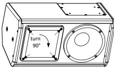
2) Unscrew the 4 screws fixing the horn and rotate the horn by 90°.
