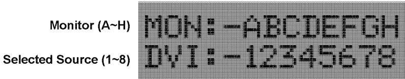
Monitor Output's are labeled 1 through 8 on the rear panel of the 8x8 DVI Matrix. These numbers correspond to the letters A through H on the LED Status Display. The top row of letters will remain static while each input number below will represent which source each of the displays are currently viewing.
