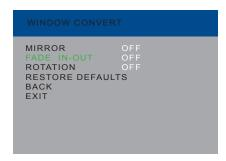
8. Use the ◀ or ▶ buttons to switch the fade feature On or Off.
