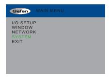
Press the Select button to display the System menu. If using the IR remote, press the OK button.
