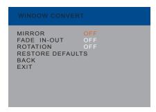
7. Use the ◀ or ▶ buttons to switch mirroring On or Off.
