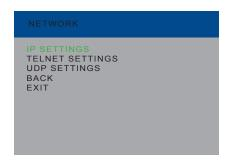
Press the Enter button again to display the IP Settings menu. If using the IR remote, press the OK button.
