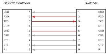
Only TXD, RXD, and GND pins are used.
