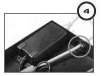
Run all connector cables out through the back of the unit. Use the included split grommets to protect the cables, as shown in the photo below:
