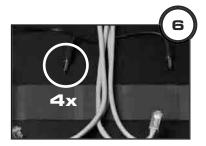
The Rack Tray provides four (4) 2.5 mm 5V DC power connectors that connect to the Gefen locking power connectors. If the device being used has 2.1 mm non-locking power connectors, then the included adapters must be used.
