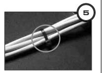
Use the included cable ties to bundle multiple smaller cords (e.g. CAT-5, CAT-6, USB, etc) and run them out through the back of the unit.
