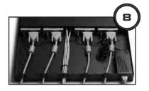
Reattach the clamping plate to the Rack Tray to secure each unit in place.
