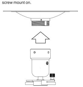
Attach security screw through hole in mount and notch in tube. For flush look, rotate mount counter-clockwise until top of mount is flush with bottom of ceiling plate. Next attach mount assembly to joist in ceiling according to instructions included in ceiling plate mount.
