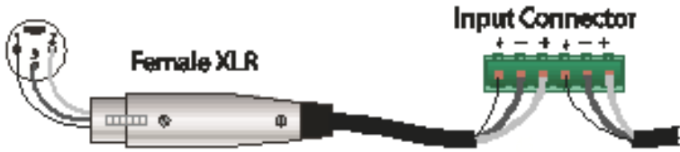
Figure 3: Connecting a Balanced XLR Input
