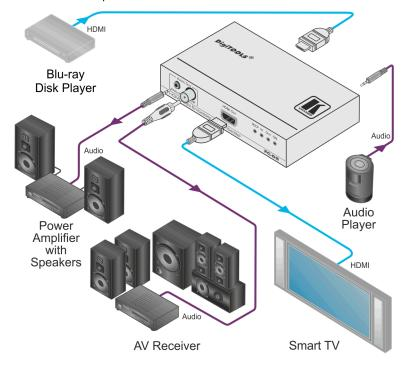
Figure 3: Connecting the FC-69 HDMI Audio Embedder/De-Embedder
