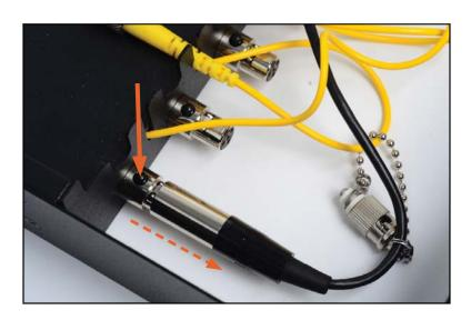
6. Use one of the included male-to-male BNC adapters and attach it to the BNC input connector of the Sender unit. Note that one end of the BNC adapter is shorter than the other. Make sure that the short end is inserted in the input on the Sender unit, as shown below. Make sure that the BNC adapter locks into place (see photo inset).
