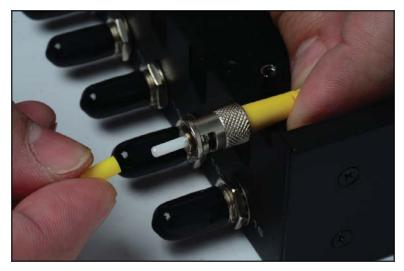
3. Connect the yellow fiber optic cable to the output connector of the 3GSDI Fiber Optic Extender Sender unit.
