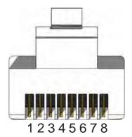
CAT-5, CAT-5e, and CAT-6 cabling comes in stranded and solid core types. Gefen recommends using solid core cabling. CAT-6 cable is also recommended.
