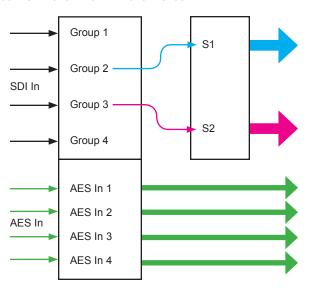
4. Use the #ch\_sw command to select which source audio channels (S1.1 ... S1.4, S2.1 ... S2.4) and/or AES audio channels (A.1 ... A.8) are routed to the output audio channels (O1.1 ... O1.4, O2.1 ... O2.4).
