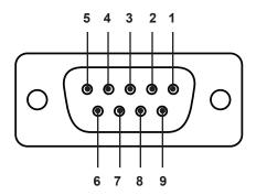
RS-232 Controller Embedder DCD 1 DCD RXD 2 RXD TXD 3 3 TXD DTR DTR 4 4 GND 5 5 GND DSR 6 6 DSR RTS 7 7 RTS CTS 8 8 CTS R1 9 9 R1
