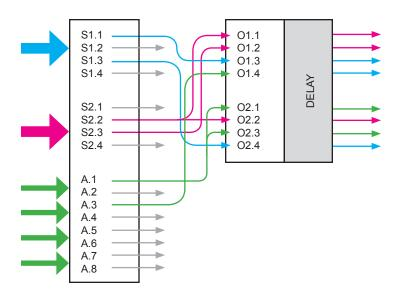
According to the block diagram on page 8, each *source audio channel* is routed to an associated *output audio channel* (S1.1 > O1.1, S1.2 > O1.2, etc). This is the default setting. If we had not allocated each *output audio channel* (O1.1 ... O2.4), the default routing (indicated by the dashed lines) would have been applied to each source channel (S1.1 ... S2.4). The diagram, below, shows the default routing state applied to O1.1, O1.4, O2.1, and O2.2.
