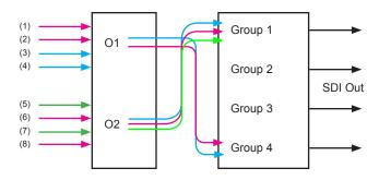
The numbers next to each arrow indicate the audio channel number. See the Audio Mapping table below for information on the channel placement.
