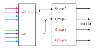
Therefore, in our example, O2 cannot be directly routed to Group 1. O2 must first be re-routed to an unused Group (highlighted in red), even if it is temporary.
