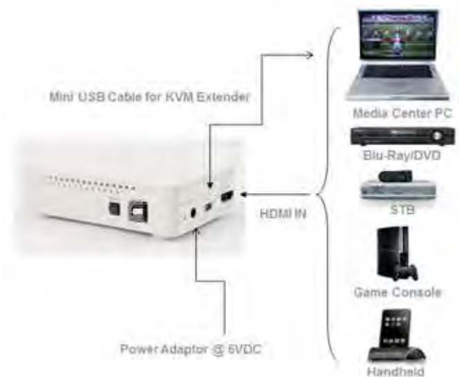
Fig. 1: Configuration of Transmitter, HDWX-100-T
