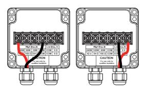
Above image indicates an example for both a 100V (left side) and low impedance (right side) connection example.
