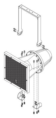
The mounting bracket includes all parts as listed below. Make sure all these parts are included with the delivery to ensure a safe and secure mounting of the loudspeaker.
