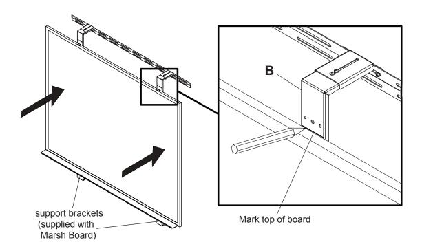
Fasten two support brackets (supplied with Marsh Board) to vertical supports (**B**) using four M5 x 12 mm phillips screws (**K**) and M5 serrated flanged lock nuts (**J**) as shown below.
