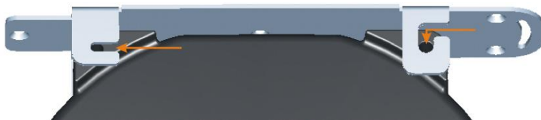
Figure 7: Inserting the Pin and Bolt into the Bracket
