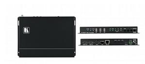
KDS-8F is a high-performance, zero latency, 4K@60Hz (4:4:4) video streaming transceiver for streaming via Ethernet over single-mode and multi-mode optical fiber. KDS-8F can be set as either an encoder or decoder. As an encoder, it encodes and streams the HDMI or DisplayPort input along with IR, RS-232, analog audio and USB, over an IP network. As a decoder, it receives the encoded signal and decodes it for output
