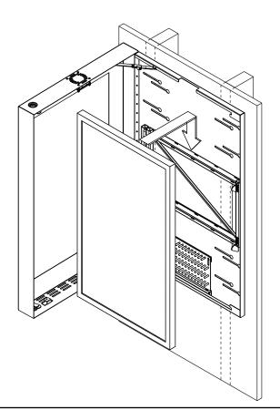
ENG Note: Mounting Arm swings out to access adapter brackets and behind display
