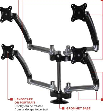
LIMITLESS POSITIONING Each arm has 12.6" of height adjustment, 22" of extension adjustment, +45/-90° of tilt, 180° of swivel and 360° of rotation
