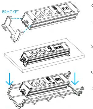
**OPTION 1 - Fix the module onto a flat surface**
