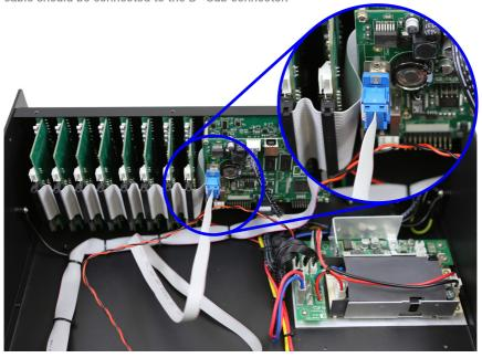
Step 13: Place and fasten the power and communication cable together with the other cables
