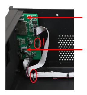
**Step 4:** Remove the 4 screws holding the dummy–plate and take–out the dummy plate.
