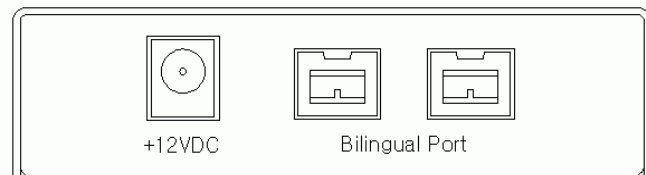
Figure 3 – Side View of M4-200 Repeater
