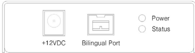
Figure 3 – Side View of M4-201 Repeater
