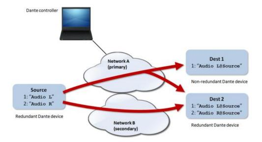
**Note:** in this mode, if (by mistake) the primary and secondary ports connect to the same Ethernet network, Dante Controller will no longer have access to the network configuration control and routing Dante<sup>™</sup> of the MIMO7272DN ports. This control is recovered when one of them is disconnected from the same network as the other.
