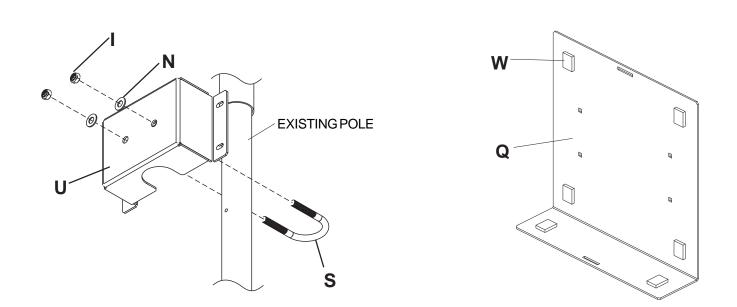
Attach PC bracket (Q) to PC mounting bracket (U) using four 1/4-20 nylock nuts (T) and four 1/4-20 x 5/8" carraige bolts (Y).
