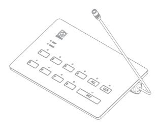
The front panel of the MPX contains various selectors and indicators. All selection buttons are implemented using capacitive touch principle, whereby selection is done by gliding your finger over it.
