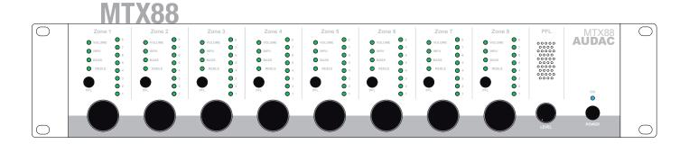
The front panel of the MTX enables you to fully control and configure the settings of every output zone. Every output zone contains its own specific control section, including one rotary function dial, four function indication LED's, and eight level / selection indication LED's.
