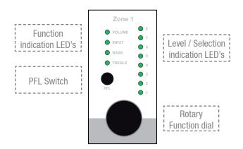
By means of the function indication LED's, the current operating function will be indicated. The upper LED stands for volume adjustment, the second LED stands for input channel selection, the third LED will blink when Bass tone adjustment is enabled, and the fourth LED will blink when Treble tone adjustment is enabled.
