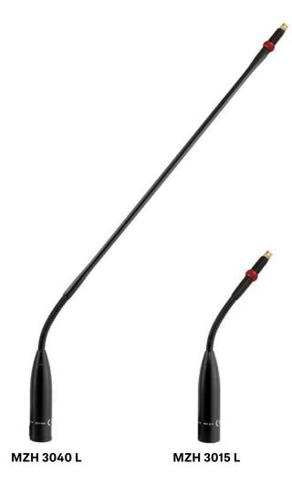
The MZH 3015 L and MZH 3040 L are sturdy and elegant metal goosenecks with one flexible element for use with the ME 34, ME 35 and ME 36 microphone capsules. The LED light ring indicates an active microphone. The rugged, matte black goosenecks are fitted with a balanced floating XLR-5M connector, enabling the microphone to be powered from 12 - 48V phantom power. Two pins are dedicated for power supply of the LED ring.
