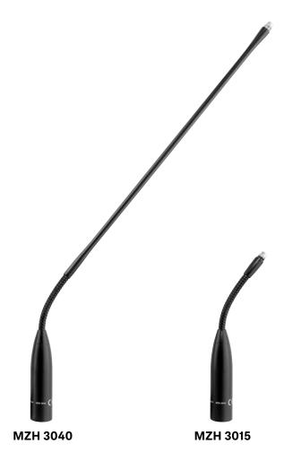
The MZH 3015 and MZH 3040 are sturdy and elegant metal goosenecks for use with the ME 34, ME 35 and ME 36 microphone heads. The rugged, matte black goosenecks are fitted with a balanced, floating XLR-3 output, enabling the microphone to be powered from 12 – 48 V phantom power.
