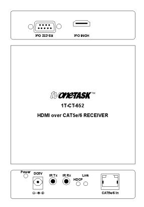
1. At the remote location, connect the Cat.5e/Cat.6 cable to the Receiver's RJ45 connector. Ensure that the connector achieves a positive lock into the receiver's connector.
