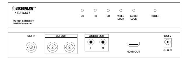
Connect the SDI source device's output to the SDI IN connector of the 1T-FC-677, using an appropriate high quality cable.
