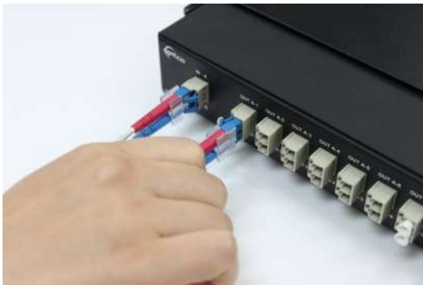
Fig. 8: LC patch cord into output receptacle
