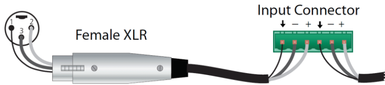
Figure 3: Connecting a Balanced XLR Input
