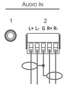
Figure 5: Connecting a Balanced Stereo Audio Source to the Balanced Input
