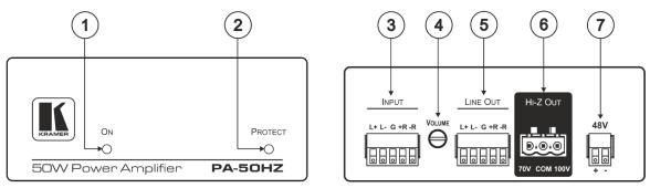
Figure 1: PA-50HZ Front and Back Panel
