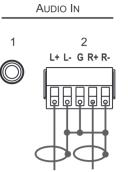
Figure 6: Connecting an Unbalanced Stereo Audio Source to the Balanced Input
