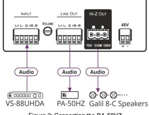
Figure 2: Connecting the PA-50HZ
