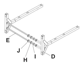
Place horizontal tube supports (**B**) between screen mount tubes (**A and B**). Attach horizontal tubes (**E**) using sixteen 1/4-20 x 1/2" phillips screws (**J**), 1/4"SAE flat washers (**I**) and 1/4" split washers (**H**).
