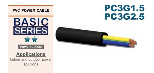
The PC3G15 and PC3G25 are high quality standard H05VV-F power cables for indoor and outdoor, fixed or mobile use. The cables are made of 3 PVC insulated conductors, with a diameter of 3 mm each (PC3G15) or 3,5 mm each (PC3G25) . These cables can be used in damp spaces.
