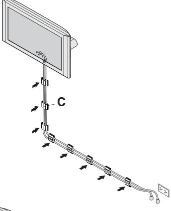
Attach covers (A) to mounting bases (C) by guiding cover flanges on covers into slide channels of mounting bases.
