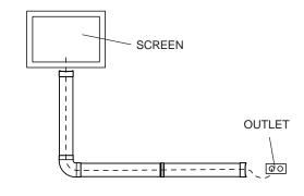
Using a level, draw a vertical line indicating the center of the covers in the vertical orientation. Mark mounting holes on the centerline down the length of covers (if covers
