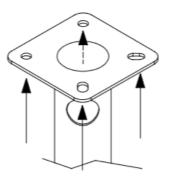
4. Screw the loudspeaker wall-mount brackets to the PCS124. It will be necessary 2 screws M6x30 for the AUDEO103 or AUDEO106 (left), or 3 screws M5x30 for the eMOTUS wall-mount bracket (right).
