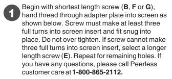
**NOTE:** Spacer (**H**) is only to be used with M8 x 25 mm socket pin screw (**G**). #10 washer (**I**) is used with M5 x 12 mm socket pin screw (**B**) only.
